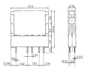
• PC board mounting hole layout (BOTTOM VIEW)
